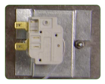
Connect the two wires\* coming off of the header with female Faston to the high-limit thermostat. See figure 3.
