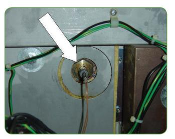
Using the included adjustment gauge (see Figure 4), insert the new probe until it reaches the gauge limit.
