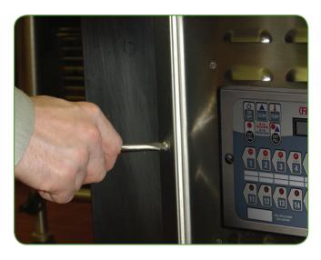
10. Plug the VC-210 harness connectors into the header assembly and secure to the header using the 2 screws provided on the controller.
