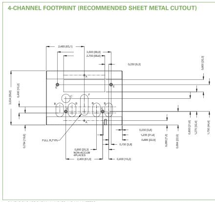
DIMENSIONS ARE SHOWN IN INCHES AND MILLIMETERS
