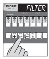
If the controller is programmed for filter lockout, FILTER will appear in the display after the pre-programmed number of cook cycles allowed. The controller will stop operating until the fryer is filtered. After filtering, the display will read FILL. **At this time, the fryer MUST be refilled with oil**. When this step is complete, press ENTER to resume normal operations.
